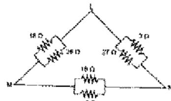
3. Obtain the maximum power transferred to R<sub>2</sub> in the circuit and also the value of R<sub>2</sub>.
