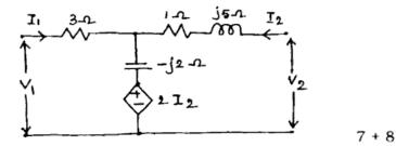
For the circuit shown in fig., find the value of Z that will receive maximum power. Also determine this power:
