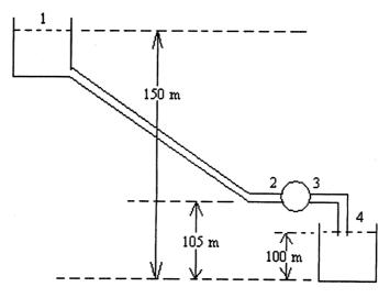
Also calculate the power generated by the turbine.
