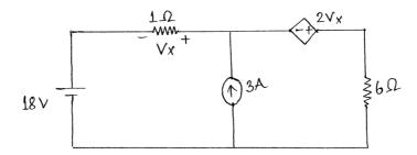
b) Find the load impedance  $Z_L$  to transfer maximum power in the circuit shown. Find also the value of maximum power consumed by the load.
