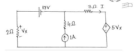
4. For the network shown in the figure, draw the oriented graph and write the incidence matrix, tie-set matrix.
