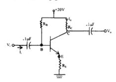
Calculate the input and output impedance and voltage gain by the amplifier. Give the de load line and the Q-point of the circuit.
